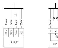
Connecting humidity sensor or CO<sub>2</sub> sensor to the control unit via a cable, which is attached to the bracket
