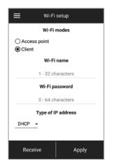
**Client** – the unit operates on the home router network. Enter the home router details and the IP address type for the **Client** mode: Enter the name of the Wi-Fi home router access point. Enter the password for the Wi-Fi home router access point. Select an IP address type:
