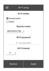
Access Point: access point mode without a home router. Up to 8 devices can be connected to the unit in this mode. Select the desired security level for the Access point mode: Open: without a password. WPA PSK: password-protected. WPA2 PSK: password-protected. WPA/WPA2 PSK: password-protected (recommended).
