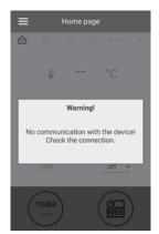
After installing the application, connect the mobile device to the unit as to a Wi-Fi access point (**FAN: + 16 characters of the ID number**) indicated on the control board and on the unit casing.
