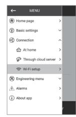
Then press **Receive**. The screen will display the current Wi-Fi parameter settings. Select one of the Wi-Fi operation modes: **Access Point** or **Client**.
