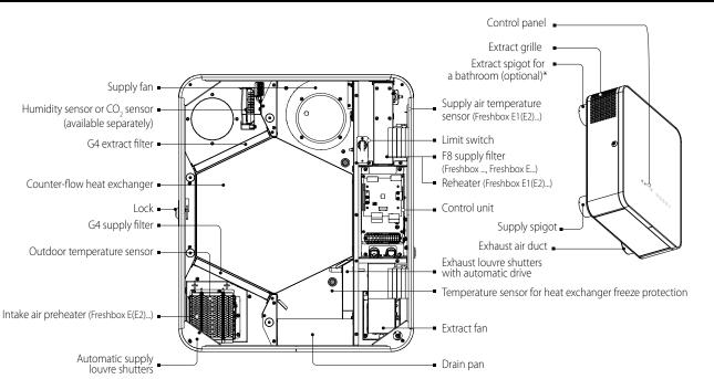
Warm stale extract air from the room flows to the unit, where it is filtered by the extract filter, then air flows through the heat exchanger and is exhausted outside by the extract fan.
